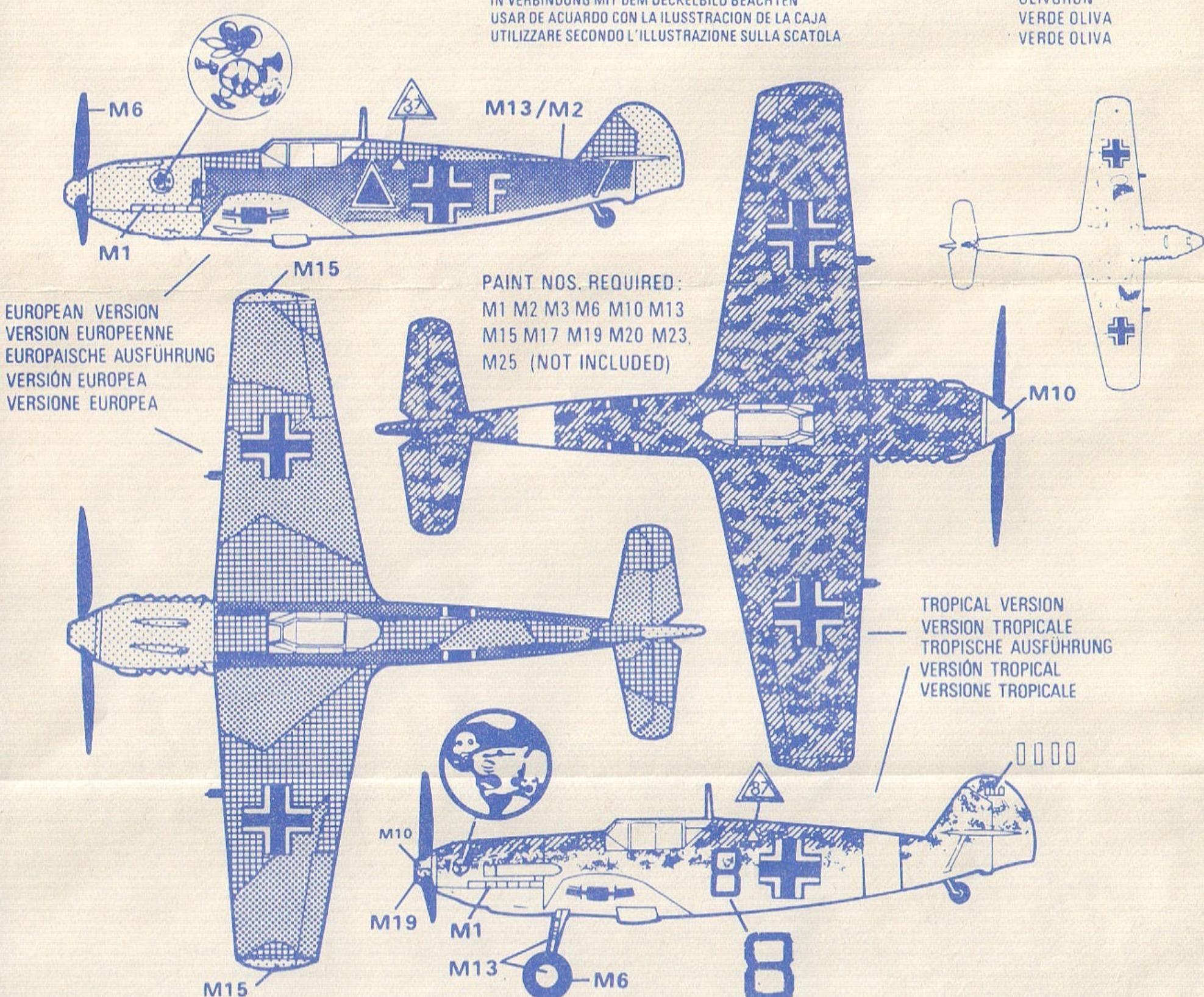
Apply transfers, separate into required subjects dip in warm water for a few seconds, slide off backing into position shown in illustration.
