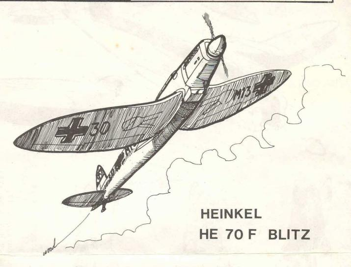
The He 70 was originally designed as a small capacity airliner and was inspired by the Lockheed Orion. It was a revolutionary design for its time, in that its lines and construction were exceptionally clean. After setting many records for speed and capacity the He 70's military potential was realised and the design altered to fill such a role. The "Blitz" made its combat debut in the Spanish Civil War as a reconnaissance aircraft, being later replaced by Do 17 s.
