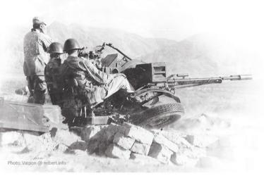
The ZU-23-2 (USSR GRAU index 2A13) is a 23-mm twin anti-aircraft gun developed in the late 1950s and adopted in 1960. It is designed to engage low-flying air targets, such as aircraft and helicopters, as well as enemy ground vehicles and manpower.
