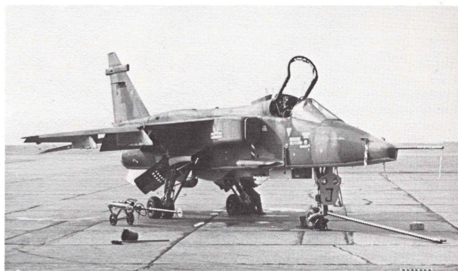
Jaguar GR1, XX764 'J' of 14 Sqn., at its home base of Bruggen, summer 1975. In this case, all undercarriage doors are opened, and when 'at rest' the air brakes are open. All Jaguar GR1's in RAF Germany have the laser nose. Although matt painted there is a noticeable sheen to the finish. Photo: C. F. Smedley.
