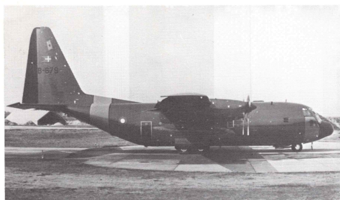
C-130H, B-679, at its home base of Vaerlose, late 1975. Note the wingtip fuel jettison pipe. The apparent fairing on top of the fuselage, just ahead of the propellers, is in fact the top of a building behind the machine; do not add this to your model! Photo: B. Mikkelsen.
