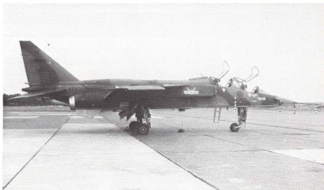
14 Sqn's Jaguar T2, XX836, at Bruggen. There are small white blade aerials above the starboard and below the port wingtips. XX836 was not given a letter code, and recently the squadron has reverted to using number codes ('last three' of the serials) in place of letters. Note the drooped leading edge slats. Photo: C. F. Smedley.
