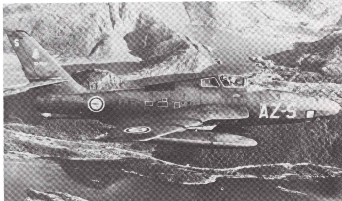
RF-84F Thunderflash, 52-7332 'AZ-S' of 717 Sqn., R. Norwegian Air Force. In this case the camera windows have been sealed over. It should be noted that all camouflaged Norwegian RF-84F's were in grey/green scheme, never in a single-tone grey or a PRU blue that some references have stated. Photo: K. Arveng, via S. Meum.
