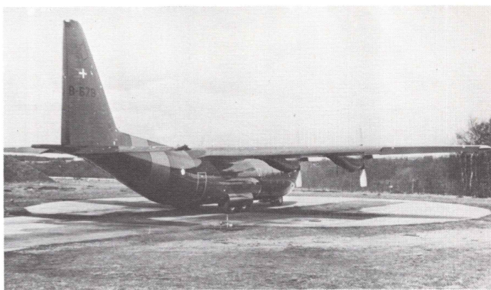
The same machine from three-quarter rear. Note that the wing trailing edge fillet is longer than in the kit, and that these machines have a high gloss finish, unlike many other R. Danish Air Force combat types. Photo: B. Mikkelsen.
