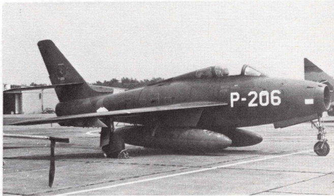
Starboard view of P-206 on the same day. Note the very weathered and different appearance between the large underwing tanks, which are of a different style to those in the kits, and lack fins. At one time, the intake rim of P-206 was believed to be painted yellow.
