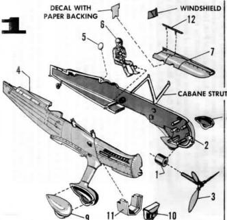
Cement propeller bearing 1 between locating pins in nose of left fuselage half 2. Paint propeller 3, see "Painting" instructions on last page. After paint has dried, insert propeller shaft through bearing and flare end with the heated blade of an old knife.
