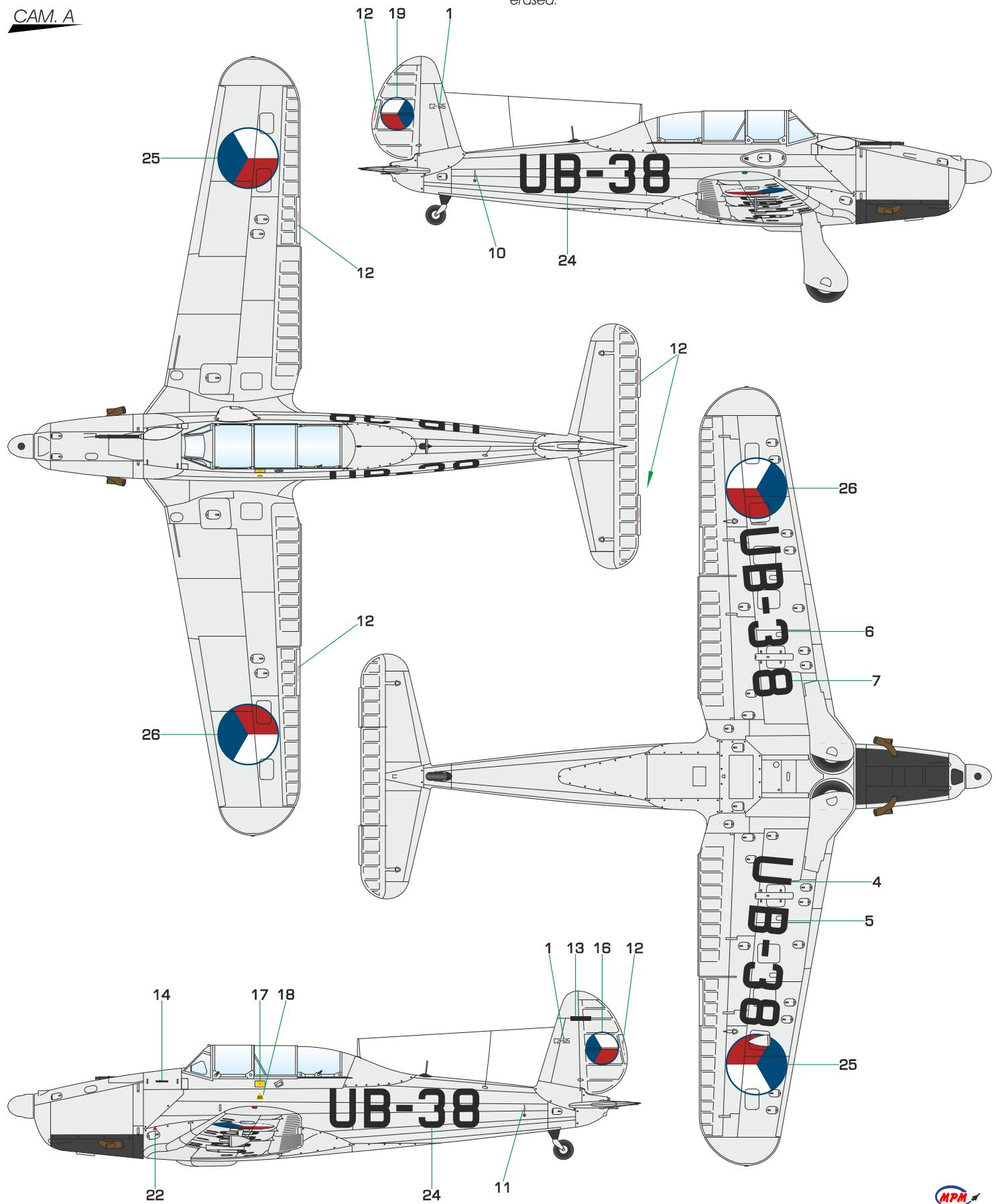
Avia C.2-615, UB-38, Letecké Učiliště (Aviation School) Prostějov, or PŠ-II Přešťany, 1950. This machine produced by Letov Company was equipped with machinegun, gun camera and Letov propeller with smooth skin spinner. The fuselage code letters were repeated on the wing lower side. According to the regulation issued on April 1, 1951 all lower side wing codes had to be erased.
