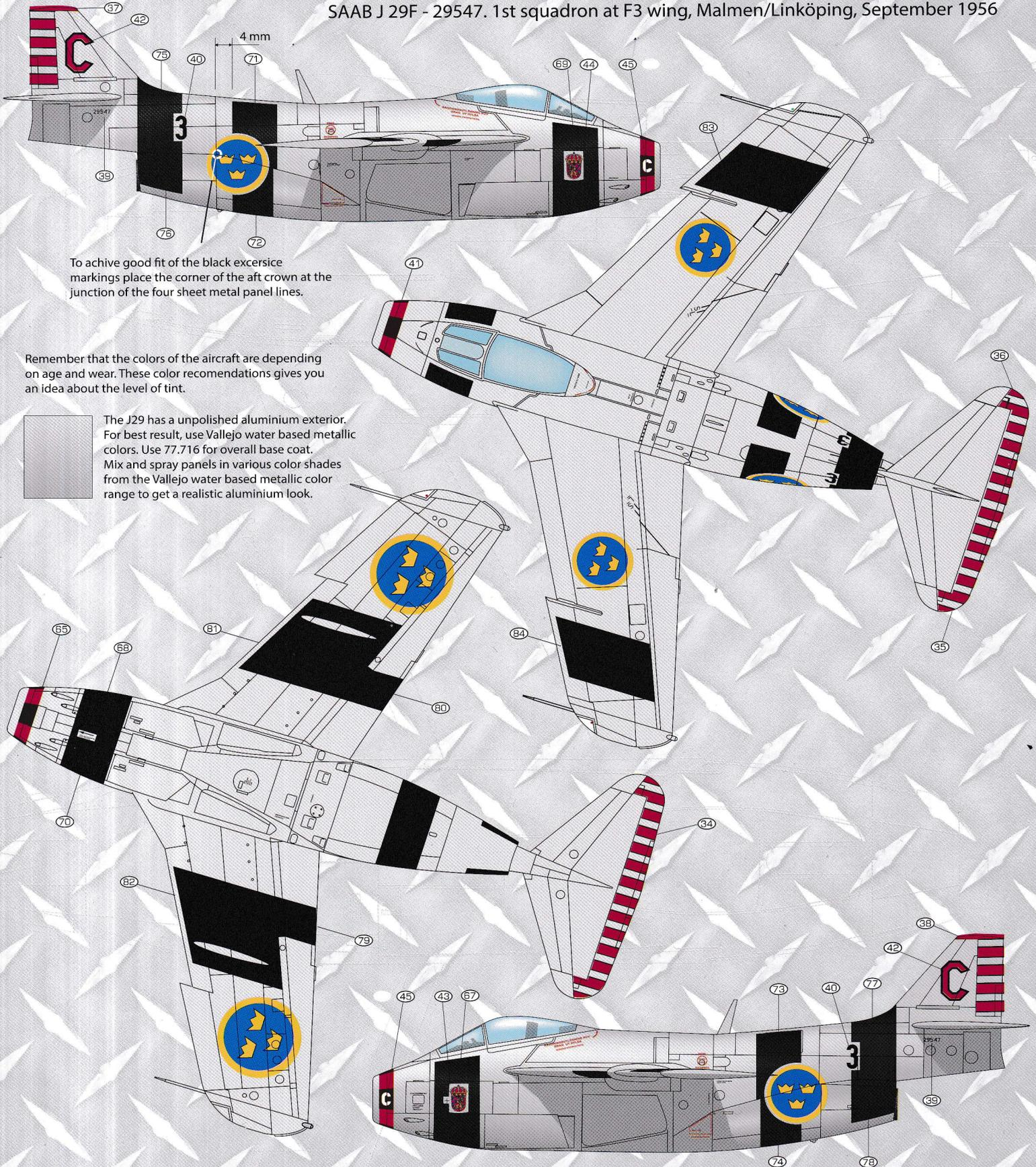
To achieve good fit of the black excersice markings place the corner of the aft crown at the junction of the four sheet metal panel lines.
