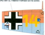
The style of \*14" on the left fuselage side is slightly different from that of A/C #2. There is a white marking on wing tips, and yellow paint is applied on lower part of engine pannier only, and lubricant oil stencil is applied on RLM78 background (confirmed by changing the photo in ref. 10 to negative). White anti-heat paint is applied to tail wheel only. Red primer paint was applied around the tail light. It seems that stencils of jack-up point and wheel pressure are aligned side by side.
